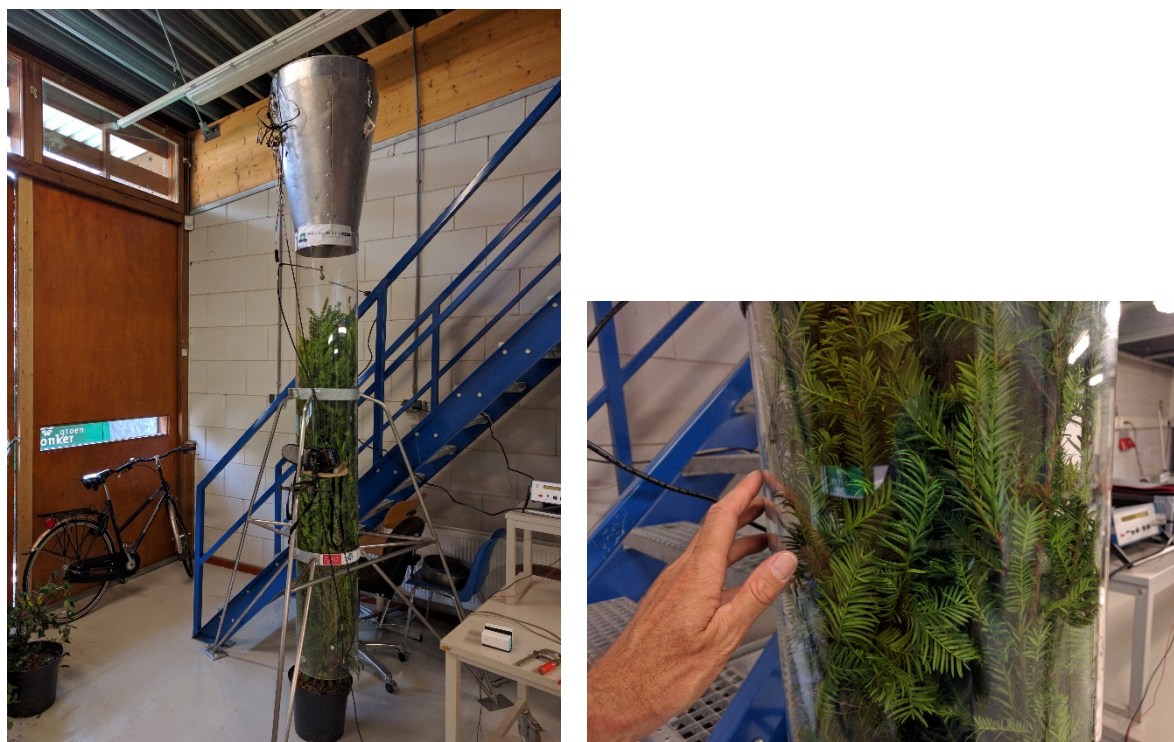
Figure 11: Taxus, high density packing and low flow rate (0.07 m/s).
