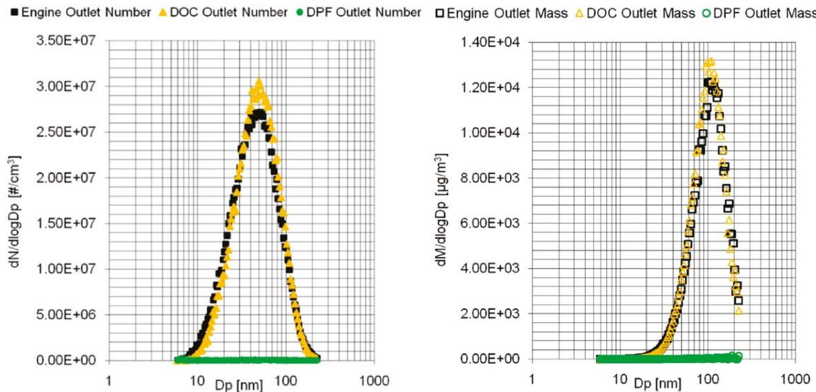
Figure 1: Diesel engine particle size number and mass distributions (Adapted from Caroca et al., 2010).
