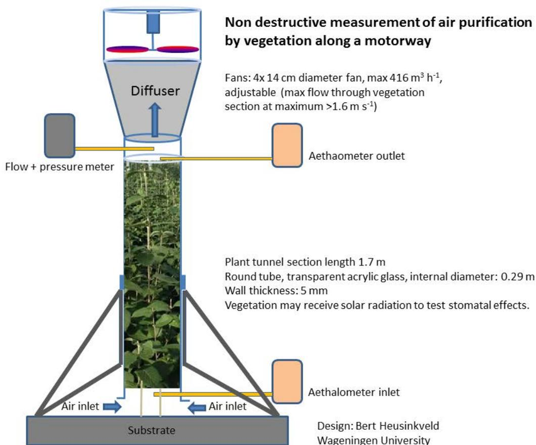
Figure 6: Schematic overview of the wind tunnel design.
