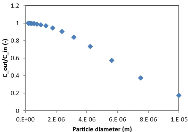
Figure 4: Simulation of the ratio of fine dust concentration output over input concentration, filter fibre diameter 20  $\mu\text{m}$ , flow 0.1 m/s and a packing density resulting in a pressure drop of 2 Pa.
